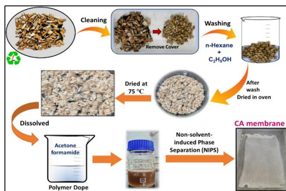
Fig. Diagram showing the entire procedure for creating CA membranes from cigarette butts using the phase inversion method
